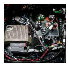
The electrical system uses Deutsch connectors, electronic fuses and relays to ensure good connectivity in the electrical system.
