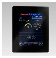
Display. The control panel display monitors engine and hydraulic functions. It allows the operator to make individual settings for crane speed, engine operating rpm and so forth. Because control panel display location is flexible, it can be installed anywhere in the driver's cab.
