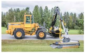
SLAGKRAFT ROAD CLEARANCE SYSTEMS No matter which solution you choose, our product systems are built with you - the operator – in mind.. The location of the cutting head means great workplace visibility; the entire machine is manoeuvred smoothly by joystick, and there's a door microswitch to ensure operator safety. These are just a few examples of how we create products for operators who demand reliable, easily manoeuvred road clearance technology.
