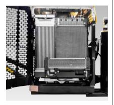
Radiator. The Craft W10 has side-by-side radiators. This makes cleaning and servicing easier.
