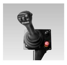
Joystick. The machine's crane and flail are controlled by a joystick. This makes it easier for the operator, who keeps one hand on the steering wheel and manoeuvres the machine with the other hand. The starter switch and emergency stop are both installed next to the joystick. A driver's cab door switch is fitted for greater safety.
