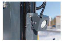
**Lights.** One LED-light is located on the cover for the lift cylinder of the crane.
