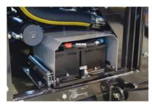
**Batteries.** W180 is equipped with a package of twin batteries. The package is mounted on a sliding shelf for easy access.
