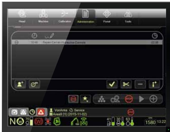
A working mode adapted to HMI (Human Machine Interaction) is provided, with various tabs that can show current production, operational monitoring information, machine alarms and much more. The modern working mode features a colour palette, contrasting elements and opti-
